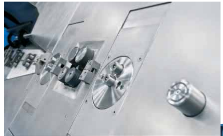
2 bending heads integrated right after the shear, for single and double bending
