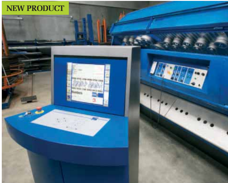
Automatic straightening units, control panel and separate PC control
