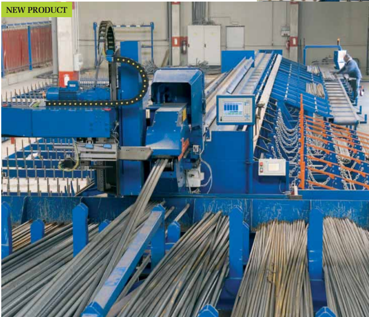
Autender S for the Combiline shearing system connected to a B-Master
