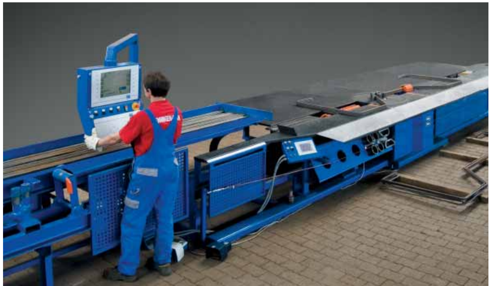
The B-Master automatic bender consists of an in-feed conveyor complete with a guide-system and support rollers
